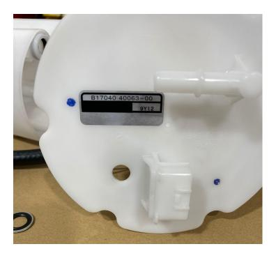
9. Make sure both surfaces are smooth and clean and place the bulkhead fitting with one of the sealing washers down through your hole oriented away from the electrical connector. Feed the other sealing washer up from the bottom and secure the fitting with the included nut.
