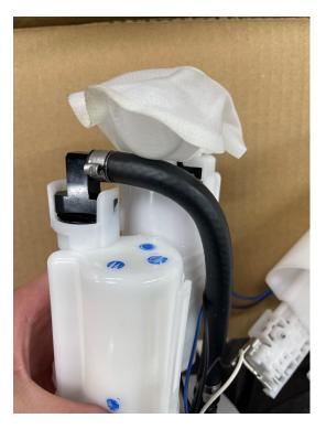
12. All of the modifications to your sending unit are done! You can carefully reinsert the main body into the basket until the small plastic tab clicks into place. It may be necessary to mess with the routing of the wires and the new return line to get everything seated and happy.
