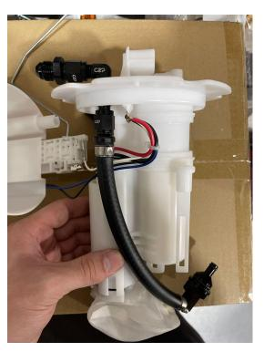
11. Make sure the o-rings are on the pressure regulator delete fitting and are well lubed. Take the delete fitting and install it into the port we took the fuel pressure regulator out of. There should be a satisfying click as the regulator clips into place.
