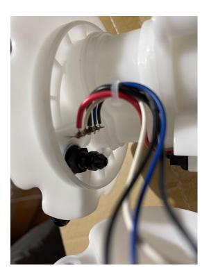
10. Now take your pressure regulator delete line and screw the -4AN female end to the bottom of the bulkhead fitting we just tightened down
