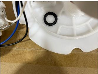
6. Besides grinding the webbing on the bottom of the hat we have to remove the majority of the three ribs on the side of the canister so our return line has room to squeeze in and not obstruct the basket from fitting and moving freely.
